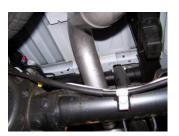
**5.** Install overaxle tailpipe #C into muffler  $1 \frac{1}{2}'' - 2''$ . Use clamp #F to secure pipe to muffler. Do not tighten.
