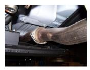
**2.** To remove stock exhaust unbolt it from the 2 bolt flange located in front of your stock muffler. You will reuse the factory nuts. Cut your stock tailpipe off for easier removal of stock exhaust. Use WD-40 to disengage hangers from rubber grommets. Do not damage or remove the rubber grommets as you will reuse them to mount your new system.
