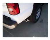
7. Install stainless steel tip #E. Clamp down. When you have everything in place, firmly tighten all bolts and clamps down securely. Use stainless steel cleaner and a Scotch Brite pad weekly to prevent tip from discoloration. Inspect all fasteners after 25-50 miles of operation and re-tighten as necessary.
