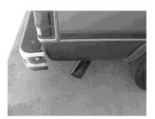
Install your Stainless Steel tip and clamp down. When you have everything in place \*, firmly tighten all your hardware and clamps securely down. To clean your stainless steel tips, use a stainless cleaner and polish.
