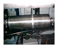
INSTALL MUFFLER #B ONTO HEADPIPE #A 1-1/2" TO 2" WITH THE LOUVERS FACING TOWARDS THE CONVERTER. USE A JACK STAND TO SUPPORT THE MUFFLER. USE CLAMP #F TO SECURE THE MUFFLER TO THE HEADPIPE. DO NOT TIGHTEN.
