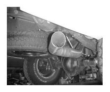
NEXT CONNECT THE TURN OUT PIPE #C TO THE OVERAXLE PIPE USING CLAMP #E. DO NOT TIGHTEN.
