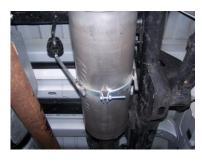
SLIDE BAND CLAMP #G ONTO MUFFLER. WITH BOLT KIT # H. INSERT HANGERS INTO RUBBER GROMMETS.
