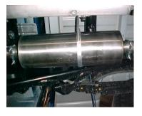
INSTALL MUFFLER #B ONTO HEADPIPE #A 1-1/2" TO 2" WITH THE LOUVERS FACING TOWARDS THE CONVERTER. USE A JACK STAND TO SUPPORT THE MUFFLER. USE CLAMP #F TO SECURE THE MUFFLER TO THE HEADPIPE. DO NOT TIGHTEN. MUFFLER INLET IS LOOKING INTO THE LOUVERS.
