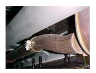
Lay out the exhaust on the floor so it looks like the drawing and compare parts with manual. To remove the stock exhaust remove it from the clamp located just in front of the muffler. You may need to heat it up for easier removal. Leave all rubber grommets in place. Use WD-40 to aid in removal of exhaust and hangers.
