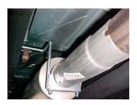
Install muffler onto head pipe # A 1-1/2" to 2" with the louvers facing towards the converter. Use a jack stand to support the muffler. Use clamp #F to secure the muffler to the head pipe. Do not tighten. Insert hanger into rubber grommet. Muffler inlet is looking into the louvers.
