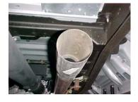
Install head pipe # A on to your existing stock front pipe and secure with clamp # I. Do not tighten.
