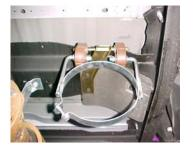
Install band clamp # F into rubber grommets located just above the axle. Do not tighten. And attach with bolt kit # I.
