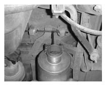
4. Slide muffler # B with inside louvers facing towards the converter. Use a jack stand to support the muffler. Install hanger # G on the muffler outlet. The long portion of the hanger will be pointing towards the driver side. Now, install rear hanger # H with hanger bolts facing towards the passenger side. Install over axle pipe # C into the outlet of muffler no less than 1 ½" and no more than 2". Do not tighten hangers.
