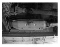
2. Remove stock exhaust from behind the catalytic converter. For easier removal cut overaxle just behind the muffler. Use jack stands to support the converter. You will want to keep the converter supported so it wont drop.
