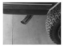
6. Install stainless steel tip, Clamp down. To clean stainless tip use any stainless steel or aluminum cleaner. When you have everything in place, make sure you have a 1" clearance on all pipes from all rubber brake lines, shock boots, tires, etc. Tighten all bolts and clamp down.
