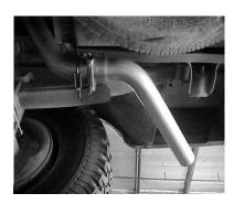
5. Slide turn out pipe # D on the tailpipe behind the rear tire. Roll turnout pipe until you have it at the correct angle for your truck and clamp # H. Spare tire may need to be loosened and pushed to the rear to allow for clearance.
