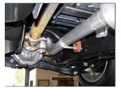
**4** Install the overaxle tailpipe #C into the muffler 1½-2". Use clamp #F to secure pipe together. DO NOT TIGHTEN. Insert welded hanger into rubber grommet.
