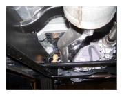
**2.** Bolt head pipe #A onto your existing stock front pipe using your stock bolts. DO NOT TIGHTEN. Insert welded hangers into rubber grommets.
