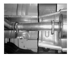
INSTALL HEADPIPE #A AND CONNECT TO STOCK EXTENSION PIPE USING CLAMP #G. DO NOT TIGHTEN. INSTALL MUFFLER OVER HEADPIPE 1½" TO 2". OUTLET OF MUFFLER WILL BE POSITIONED AT ABOUT 7 TO 8:00 O'CLOCK. USE CLAMP #F TO ATTACH MUFFLER TO HEADPIPE. THE MUFFLER INLET IS LOOKING INTO THE LOUVERS. USE A JACKSTAND TO SUPPORT MUFFLER.
