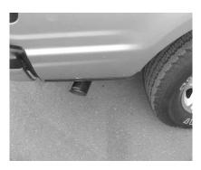
INSTALL STAINLESS STEEL TIP. USE ANY ALUMINUM OR STAINLESS STEEL CLEANER TO POLISH YOUR TIP. NOW FIRMLY TIGHTEN ALL CLAMPS AND HANGERS.
