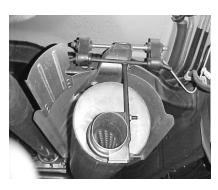
INSTALL HANGER #H ONTO THE MUFFLER OUTLET AND INSERT ROD INTO GROMMETS. THE VERTICAL ROD WILL BE ON THE PASSENGER SIDE OF OUTLET. DO NOT TIGHTEN.
