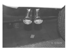
Install the passenger side over axle tailpipe #C onto muffler at least 1-1/2" to 2" using clamp #F to attach tailpipe. Insert welded hanger into rubber grommet. Do not tighten. Install Driver side over axle tailpipe #D into muffler at least 1-1/2" to 2" using clamp #F to attach tailpipe. Install hanger #G onto driverside tailpipe and insert into rubber grommet. Use Bolt Kit #H to secure both tailpipes together.
