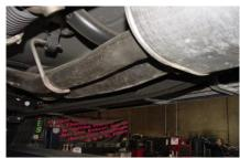
TO REMOVE STOCK EXHAUST, CUT 13" FROM THE FRONT OF THE MUFFLER, MEASURE TOWARDS THE FRONT OF THE VEHICLE. LEAVE ALL RUBBER GROMMETS ON THE HANGERS. USE WD-40 TO AID IN THE REMOVAL OF EXHAUST AND HANGERS. SUPPORT THE CATALITIC CONVERTER BEFORE CUTTING.
