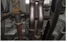
SLIDE PASSENGER SIDE HEADPIPE #A ONTO STOCK HEADPIPE. INSERT WELDED HANGER INTO RUBBER GROMMET. NEXT INSTALL DRIVERS SIDE HEADPIPE #B ONTO STOCK HEADPIPE, USE CLAMP #G TO SECURE BOTH HEADPIPES, DO NOT TIGHTEN.
