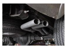
USE BOLT KIT #J TO SECURE TAILPIPES TOGETHER. THE PASSENGER SIDE TAILPIPE WILL BE ON THE BOTTOM.
