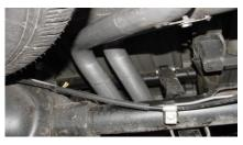
SLIDE PASSENGER SIDE TAILPIPE #E INTO MUFFLER 1-1/2" TO 2". USE CLAMP #I TO SECURE TAILPIPE TO MUFFLER. DO NOT TIGHTEN.
