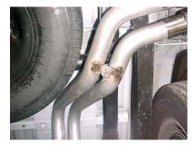
BOLT THESE TOGETHER USING BOLT KIT #H.
