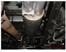
SLIDE MUFFLER #C ONTO HEADPIPES 1-1/2" TO 2". OUTLETS SHOULD BE AT THE BOTTOM. USE A JACK STAND TO SUPPORT MUFFLER. ATTACH TO HEADPIPES WITH CLAMP #G.
