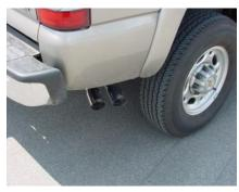
**INSTALL YOUR** STAINLESS STEEL TIPS. TO CLEAN TIPS USE A SCOTCH BRITE PAD AND ANY STAINLESS OR ALUMINUM CLEANER. AFTER YOU HAVE CHECKED FOR **CLEARANCES GO BACK AND** TIGHTEN ALL **NUTS, BOLTS AND** CLAMPS.
