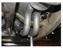
SLIDE PASSENGER SIDE HEADPIPE #A ONTO STOCK HEADPIPE. INSERT WELDED HANGER INTO RUBBER GROMMET. NEXT INSTALL DRIVERS SIDE HEADPIPE #B ONTO STOCK HEADPIPE, USE CLAMP #G TO SECURE BOTH HEADPIPES, DO NOT TIGHTEN.
