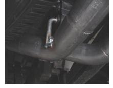
SLIDE DRIVERS SIDE TAILPIPE #D INTO MUFFLER 1-1/2" TO 2". INSERT WELDED HANGER INTO RUBBER GROMMET.
