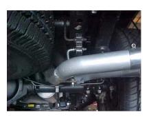
INSTALL PASSENGER SIDE TAILPIPE #D ONTO MUFFLER 1  $\frac{1}{2}$ " TO 2". USE CLAMP #G TO SECURE PIPE TO THE MUFFLER. DO NOT TIGHTEN. INSERT WELDED HANGER INTO RUBBER GROMMET.
