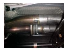
REMOVE YOUR STOCK EXHAUST FROM THE FACTORY FLANGES LOCATED JUST BEHIND YOUR FACTORY Y-PIPE. NEXT CUT OFF YOUR TAILPIPE JUST BEHIND THE MUFFLER. USE WD-40 TO AID IN THE REMOVAL OF RUBBER GROMMETS FROM HANGERS
