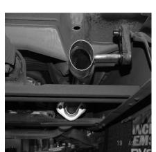
BOLT HEADPIPE #B TO STOCK FLANGE RE-USING STOCK NUTS AND BOLTS. INSERT WELDED HANGER INTO RUBBER GROMMETS.
