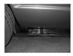
MAKE SURE YOU HAVE A 1" CLEARANCE ON ALL PIPES FROM ALL BRAKE, FUEL LINES, SHOCKS, TIRES, ETC...
