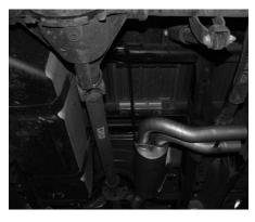
ROTATE THE MUFFLER ASSEMBLY UNTIL THE OUTLETS ARE LEVEL.
