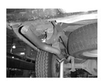
INSTALL THE EXIT PIPES #F TO YOUR DESIRED LOOK. ATTACH WITH CLAMPS #G. MAKE SURE YOU HAVE A MINIMUM OF A 1" CLEARANCE FROM ALL BRAKE LINES, TIRES, SHOCKS FUEL LINES, ETC. THEN TIGHTEN ALL CLAMPS AND HANGERS. NOW INSTALL THE STAINLESS STEEL TIPS USE SUPPLIED ZIP TIES TO TIE AWAY THE BRAKE AND FUEL LINES.
