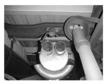
Slide muffler on 1-1/2" to 2" to headpipes and connect using clamps #G. DO NOT TIGHTEN. Level muffler outlets across at 12 o'clock position. Attach hanger #H to driverside muffler outlet and insert rod into rubber grommet.
