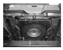
Now install exit pipes #F to tailpipe using clamp #G. Trim Exit pipes to desired length Now tighten all clamps down starting from the head pipe and working back. Re-route vent line, and tie back brake lines with zip ties. Install Stainless tins
