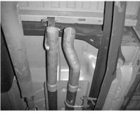
Slide head pipes #A and B over stock headpipes 1-1/2" to 2". Insert welded hanger on driver side headpipe into rubber grommet. Attach headpipe to stock headpipe with clamps #J.
