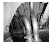
INSTALL OVERAXLE TAILPIPES # D & # E INTO THE MUFFLER USING # H CLAMP ON THE PASSENGER SIDE AND # I HANGER CLAMP ON THE DRIVER SIDE. OVERAXLE PIPES GO INTO THE REAR OF THE MUFFLER NO MORE THAN 2". LOOKING FROM THE REAR OF THE VEHICLE. THE DRIVER SIDE OVERAXLE WILL BE POSITIONED AT ABOUT 10 O'CLOCK.
