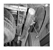
INSTALL EXIT PIPES # F ON DRIVER AND PASSENGER SIDE. USE CLAMP # H TO ATTACH BOTH PIPES TOGETHER AND TO HANGER # J 10" METAL HANGER. THE BOTTOM SECTION OF THE HANGER ROTATES IN ORDER TO ADJUST FOR CLAMPING. CUT EXIT PIPES FOR PROPER LENGTH ON YOUR VEHICLE.
