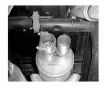
INSTALL HEADPIPES # A & # B USING CLAMP # G TO ATTACH HEADPIPES TO STOCK CONNECTOR PIPE. INSERT WELDED HANGER INTO RUBBER GROMMET. (DO NOT TIGHTEN).
