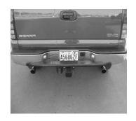
WHEN YOU HAVE EVERYTHING IN PLACE FIRMLY TIGHTEN ALL CLAMPS AND HANGERS. YOU MAY NEED TO USE THE SPARE TIRE BRACKET TO HOLD THE TIRE BACK. INSTALL IT 2" INSIDE OF THE UPPER SHOCK MOUNT ON THE DRIVER SIDE. USE ZIP TIES TO TIE AWAY BRAKE LINES. RE-INSTALL THE O2 SENSOR INTO PASSENGER HEADPIPE. USE ANTI-SEIZE ON ALL THREADS. INSTALL STAINLESS TIPS.
