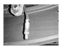
UN-BOLT THE FACTORY 02 SENSOR BEHIND THE PASSENGER CATALYTIC CONVERTER (CAREFULLY REMOVE SO NO DAMAGE OCCURS!) REMOVE THE FACTORY EXHAUST BY CUTTING 16" IN FRONT OF THE MUFFLER ON THE PASSENGER SIDE AND UN-BOLT 33" IN FRONT OF YOUR MUFFLER ON THE DRIVER SIDE HEADPIPE. FOR EASIER REMOVAL OF THE STOCK EXHAUST YOU MAY NEED TO CUT YOUR STOCK TAILPIPE BEHIND THE MUFFLER. MAKE SURE TO LEAVE ALL STOCK RUBBER MOUNTING GROMMETS IN PLACE. USE WD-40 ON ALL RUBBER GROMMETS.
