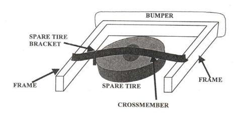
THIS SPARE BRACKET IS USED FOR BETTER CLEARANCE FROM THE SPARE TIRE. INSTALL THIS BRACKET ON THE FACTORY CROSS MEMBER LOCATED ABOVE THE SPARE TIRE. THIS BRACKET IS DESIGNED TO HOLD THE SPARE TIRE TOWARDS THE DRIVERSIDE GIVING YOU MORE CLEARANCE ON THE TAILPIPES.
