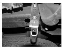
INSTALL METAL HANGERS # J INTO HOLES LOCATED APPROX.
