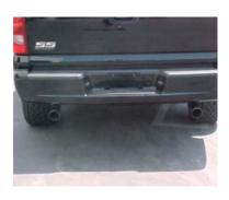
INSTALL EXIT PIPES # F ONTO TAILPIPES. CUT TO YOUR PREFERED LENGTH USE CLAMPS # I TO SECURE EXIT PIPES TO TAILPIPES. THESE CLAMPS ALSO ATTACH TO METAL HANGERS # J. THESE METAL HANGERS NEED TO BE ROTATED IN ORDER TO ADJUST FOR CLAMPING. NOW YOU CAN TIGHTEN ALL CLAMPS, NUTS, AND BOLTS. STARTING FROM THE FRONT WORKING BACK. INSTALL STAINLESS TIPS T. USE ZIP TIES FOR BRAKE AND FUEL LINES...
