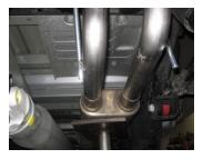
4. Install muffler #B onto head pipe #A 1.5-2" with louvers facing towards the converter. Use a jack stand to support the muffler. Use clamp #G to secure together. Do not tiahten.
