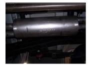
**3.** Install muffler #C onto headpipes  $1\frac{1}{2}$ "-2" with the louvers facing towards the Y-pipe. Use a jack stand to support the muffler. Use clamp #G to secure the muffler to the headpipes. DO NOT TIGHTEN.
