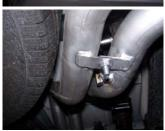
**4.** Install passenger tailpipe #D onto muffler  $1\frac{1}{2}$ "-2". Secure using clamp #G. DO NOT TIGHTEN. Insert welded hanger into rubber grommet. Next install driver tailpipe #E onto muffler  $1\frac{1}{2}$ "-2" secure using clamp #G. DO NOT TIGHTEN. Insert welded hanger into rubber grommet. Attach tailpipes with bolt kit #H with driver side tab on bottom.
