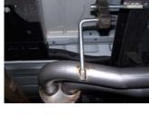
3. Attach rear hanger #H to frame with bolt kit #I just in front of crossmember. DO NOT TIGHTEN. Attach a rubber grommet off the stock hanger from the rear to the new hanger.
