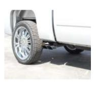
6. Install right and left stainless steel tips. Clamp down. When you have everything in place, firmly tighten all bolts and clamps down securely. Use stainless steel cleaner and a Scotch Brite pad weekly to prevent tip from discoloration. Inspect all fasteners after 25-50 miles of operation and retighten as necessary.
