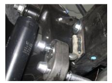
5.Next install drivers side rear hanger and gommet with bolt kit provided see picture the hanger goes on the outside of the frame and bolts through the whole frame
