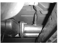
RE-INSTALL O2 SENSOR. USE A SMALL AMOUNT ANTI-SIEZE ON THE THREADS. NOW FIRMLY TIGHTEN ALL CLAMPS, HANGERS, FLANGE, AND BOLTS.
