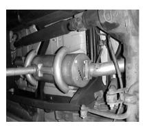
SLIDE MUFFLER #B WITH DUAL INLET ONTO HEADPIPE AT LEAST 1-1/2" TO 2". MUFFLER OUTLET SHOULD BE AT THE 12 O'CLOCK POSITION. USE CLAMPS #F TO ATTACH HEADPIPE. MAKE SURE INLETS AND MUFFLER IS LEVEL. AND TIGHTEN DOWN. USE JACK STAND TO SUPPORT MUFFLER.
