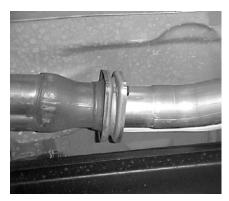
UNBOLT THE STOCK EXHAUST AT THE FLANGE BEHIND THE Y-PIPE AND REMOVE. MAKE SURE TO LEAVE ALL RUBBER GROMMETS IN THE FACTORY LOCATION. YOU WILL RE-USE STOCK NUTS AND BOLTS. FOR EASIER REMOVAL OF EXHAUST, CUT BEHIND THE MUFFLER. USE WD-40 TO REMOVE HANGERS FROM GROMMETS.
