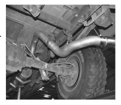
INSTALL OVERAXLE TAILPIPE #D INTO MUFFLER. INSERT WELDED HANGER INTO RUBBER GROMMET. USE CLAMP #F TO SECURE PIPE TO MUFFLER, DO NOT TIGHTEN.
