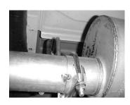
Install muffler #B onto head pipe #A 1-1/2" to 2" with the louvers facing towards the converter. Use a jack stand to support the muffler. Use clamp #G to secure the muffler to the head pipe. Insert hanger into rubber grommet. Do not tighten. Muffler inlet is looking into the louvers.
