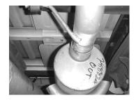
Install tailpipe # C into the muffler at least 1-1/2" to 2". Secure pipe to the muffler using clamp # E. Do not tighten. Insert welded hanger into rubber grommet.
