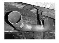
Install exit pipe #D onto the tailpipe. Insert welded hanger into rubber grommet. Secure pipes together with clamp # E. Do not tighten. Roll the exit pipe until it is at the correct angle for your truck.
