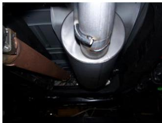
**4.** Install muffler #C onto headpipes 1 1/2"-2". Use a jack stand to support the muffler. Outlet of muffler will be at 6 o'clock position. Use clamps #F to secure the muffler to the headpipes. Do not tighten. Muffler inlet is looking into the louvers.
