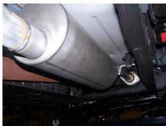
**5.** Install overaxle tailpipe #D into muffler 1 1/2"-2". Insert welded hangers into rubber grommets use clamp #G to secure tail pipe to muffler. Do not tighten.
