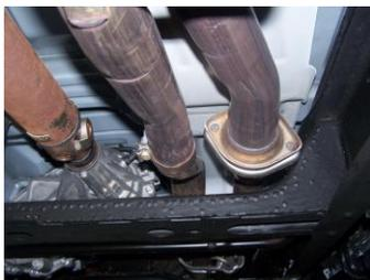
**2.** To remove the stock exhaust, remove it from the clamp on the driver side & flange on the passenger side located in front of the stock muffler. Disengage the welded hangers using WD-40 from the OEM rubber grommets. Do not damage or remove the rubber grommets as you will reuse them to mount your new system. Now, cut off tailpipe and remove exhaust.
