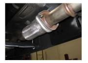
2. To remove your stock exhaust, unbolt the 2-bolt flange located in front of the muffler. Then cut off your tailpipe. Leave all rubber grommets in place. Use WD-40 to aid in the removal of the hangers from the rubber grommets.
