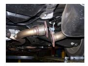
**2.** Install passenger side muffler assembly #A onto stock flange using bolt kit #C. Use a jack stand to support the muffler to insert welded hangers into rubber grommets. Insert clips onto hangers.
