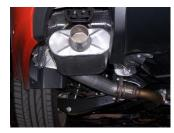
**3.** Install driver side muffler assembly #A onto stock flange using bolt kit #C. Use a jack stand to support the muffler to insert welded hangers into rubber grommets. Insert clips onto hangers.
