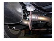
**1.** Unbolt factory muffler from flange located in front of muffler and remove. Repeat for other side. Save the stock gaskets and hardware. They will be reused.
