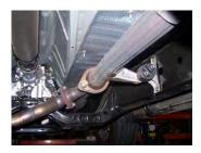
2. To remove the stock exhaust, unbolt the 2-bolt flange just in front of the muffler. Then cut your tailpipe off behind the muffler. Leave all rubber grommets on the factory hangers on the vehicle.
