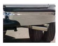
Install the over axle tailpipe # C into the muffler 1-1/2" to 2". Secure to the muffler using clamp # H Do not tighten. You may need to loosen spare tire & push over towards driverside & re tighten. Next install exit pipe # D onto overaxle pipe insert hanger into rubber grommet. Use clamp # H to secure pipes together rotate to proper angle for your vehicle. DO NOT TIGHTEN.
