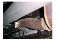
Lay out the exhaust on the floor so it looks like the drawing and compare parts with manual. To remove the stock exhaust remove it from the clamp located just in front of the muffler. You may need to heat it up for easier removal. Leave all rubber grommets in place. Use WD-40 to aid in removal of exhaust and hangers.
