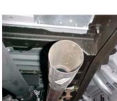
Install head pipe # A front pipe and secure with clamp # I. Do not tighten.
