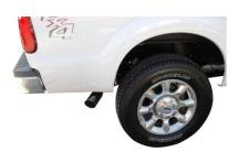
**5.** NOW INSTALL YOUR STAINLESS STEEL TIP. USE ANY ALUMINUM OR STAINLESS CLEANER TO POLISH YOUR TIP. THEN TIGHTEN ALL CLAMPS AND HANGERS.
