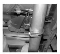
INSTALL T-HANGER # H ONTO OVERAXLE TAILPIPE AND INSERT INTO RUBBER GROMMET. THE HANGER SHOULD BE FACING TOWARDS THE DRIVERSIDE. MAKE SURE YOU HAVE EQUAL SPACE BETWEEN SHOCK AND SPARE TIRE. THE SPARE TIRE MAY NEED TO BE LOOSENED AND PUSH TO THE DRIVER SIDE AND THEN ROTATE TO GAIN CLEARANCE.
