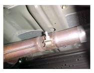
REMOVE YOUR STOCK EXHAUST FROM THE CLAMP LOCATED JUST AFTER YOUR STOCK **Y-PIPE** CUT OFF TAILPIPE JUST BEHIND THE MUFFLER USE WD-40 TO AID IN REMOVAL OF HANGER LEAVE RUBBER GROMMETS IN PLACE. NEXT, INSTALL HEADPIPE #A ONTO **Y-PIPE USING CLAMP** #F TO SECURE, DO NOT TIGHTEN.
