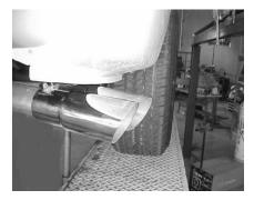
INSTALL STAINLESS STEEL TIPS. USE ANY ALUMINUM OR STAINLESS STEEL CLEANER TO POLISH TIPS. THEN TIGHTEN ALL CLAMPS AND HANGERS WATCH FOR MOVEMENT OF TAILPIPES WHEN TIGHTENING TAILPIPES.
