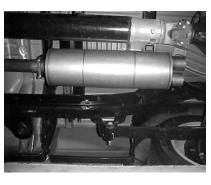
INSTALL MUFFLER # A WITH THE INLET TOWARDS THE MOTOR. INLET HAS LOUVERS INSIDE FACING TOWARDS THE MOTOR. USE A JACK STAND TO SUPPORT THE MUFFLER. USE CLAMP # F TO SECURE MUFFLER TO THE STOCK HEADPIPE. DO NOT TIGHTEN.
