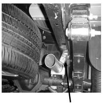
UNBOLT AND REMOVE STOCK REAR HANGER ON THE PASSENGER SIDE FRAME RAIL. INSTALL HANGERS # HTO THE BOTTOM OF FRAME RAIL IN EXISTING HOLE APPROX. 22 .5" FROM THE REAR OF THE FRAME, USE NUT AND BOLT THAT ARE SUPPLIED. REPEAT THIS SAME PROCEDURE ON DRIVERS SIDE. HANGER # H WILL AIM TOWARDS THE REAR OF THE VEHTCLE
