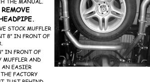
NEXT, INSTALL HANGER # G TO THE PASSENGER SIDE OF MUFFLER OUTLET WITH VERTICAL BAR OF THE HANGER TOWARDS PASSENGER SIDE INSTALL PASSENGER SIDE OVERAXLE PIPE # D INTO MUFFLER AT LEAST 1 ½" TO 2".AND USE CLAMP # F TO ATTACH... DO NOT TIGHTEN
