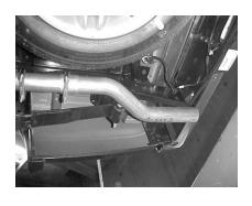
INSTALL EXIT PIPES # E TO OVERAXLE PIPES USING CLAMP # F TO SECURE THEM. DO NOT TIGHTEN, INSTALL CLAMP # F TO HANGER # H ON BOTH SIDES TO HOLD UP YOUR TAILPIPES. ADJUST PIPES TO THE RIGHT ANGLE AND CUT IF NECESSARY TO LENGTH. IF YOUR VEHICLE HAS A SWAY BAR YOU MAY HAVE TO TRIM THE FACTORY BOLT ON THE PASSENGER SIDE
