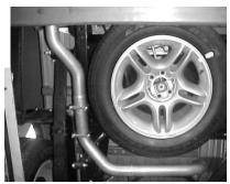
INSTALL DRIVERSIDE FRONT TAILPIPE #B INTO MUFFLER AT LEAST 1 ½" TO 2". USING CLAMP # F. NEXT INSTALL DRIVERSIDE OVERAXLE PIPE # C TO FRONT TAILPIPE USING CLAMP # F DO NOT TIGHTEN
