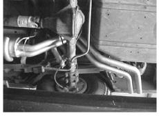
Install the passenger side over axle tailpipe #C onto muffler at least 1-1/2" to 2" using clamp #F to attach tailpipe. Do not tighten. Insert welded hanger into rubber grommet. Install Driver side over axle tailpipe #D onto Muffler at least 1-1/2" to 2" using clamp #F to attach tailpipe. Use Bolt Kit #G to secure both tailpipes together.
