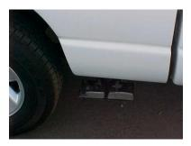
INSTALL YOUR STAINLESS TIPS # C,D. THERE IS A LEFT AND A RIGHT TIP. TIGHTEN ALL CLAMPS AFTER YOU MAKE SURE YOUR TAILPIPES ARE LEVEL.
