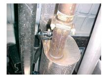
TO REMOVE STOCK **EXHAUST UNCLAMP IT** FROM THE CLAMP **LOCATED JUST IN** FRONT OF YOUR STOCK MUFFLER. DO NOT REMOVE STOCK HEADPIPE. YOU MAY NEED TO HEAT IT UP WITH A TORCH TO REMOVE IT. NOW CUT OFF YOUR STOCK TAILPIPE JUST BEHIND THE MUFFLER AND REMOVE.LEAVE ALL RUBBER GROMMETS ON THE HANGER. USE WD-40 TO AID IN **REMOVAL OF EXHAUST AND** HANGERS.
