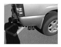
Install rear muffler hanger # H into rubber grommet located just above driverside outlet slide clamp onto muffler outlet.
