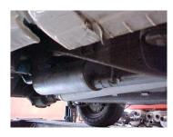
Install muffler #B onto head pipe # A 1-1/2" to 2" with the louvers facing towards the converter. Use a jack stand to support the muffler. Use clamp # G to secure the muffler to the head pipe. Do not tighten.
