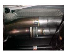
INSTALL PASSENGER SIDE HEADPIPE #A ONTO FACTORY FLANGE USING THE HARDWARE PROVIDED TO SECURE. DO NOT TIGHTEN. INSERT HANGER INTO RUBBER GROMMET. NEXT INSTALL DRIVER SIDE HEADPIPE #B ONTO THE FACTORY PIPE. USE CLAMP #G TO SECURE. DO NOT TIGHTEN.
