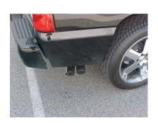
MAKE SURE YOU HAVE A 1" CLEARANCE FROM ALL BRAKE LINES, FUEL LINES, SHOCKS, TIRES, ETC.
