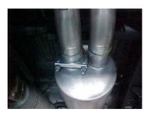
INSTALL REAR MUFFLER HANGER #H ONTO DRIVER SIDE OUTLET OF MUFFLER. INSERT HANGER INTO RUBBER GROMMET. DO NOT TIGHTEN.
