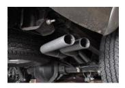
**8.** Use bolt kit #H to secure tail pipes together. The passenger side tail pipe will on the bottom.
