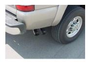
**11.** Install stainless steel tips. Clamp down. When you have everything in place, firmly tighten all bolts and clamps down securely. Use stainless steel cleaner and a Scotch Brite pad weekly to prevent tip from discoloration. Inspect all fasteners after 25-50 miles of operation and re-tighten as necessary.
