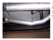
**3.** Install head pipe #A, using the two stock bolts. Insert hangers into rubber grommets. Do not tighten.
