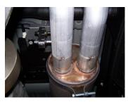
**4.** Slide muffler #B onto head pipe #A 1½"-2". Use a jack stand to support the muffler. Install band clamp #I onto muffler. Insert hanger on band clamp into rubber grommets. Use bolt kit provided. Do not tighten.
