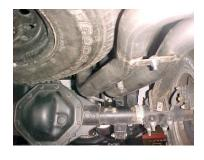
Install the driver side over axle tailpipe # C into the muffler. 1-1/2 TO 2". Use clamp #E to secure tailpipe to muffler. Do not tighten.
