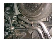
Install passenger side over axle tailpipe # B into muffler 1-1/2" – 2" and attach using clamp # E. Insert hanger into rubber grommet.
