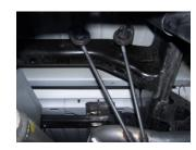
3. Insert welded hangers into rubber grommets.
