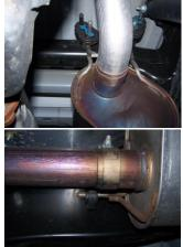
1. To remove the stock exhaust remove it from in front of the stock muffler. Disengage the welded hangers using WD-40 from the OEM rubber grommets. Do not damage or remove the rubber grommets as you will re-use them to mount your new system. Now, cut off tailpipe and remove exhaust.
