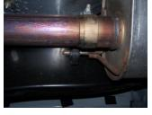
2. Insert muffler assembly #A into headpipe head pipe and attach with clamp #B. DO NOT TIGHTEN Use a jack stand to support the muffler assembly.
