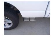
4. Install stainless steel tips. Clamp down. When you have everything in place, firmly tighten all bolts and clamps down securely. Use stainless steel cleaner and a Scotch Brite pad weekly to prevent tip from discoloration.
