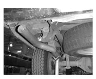
INSTALL THE EXIT PIPES #F TO YOUR DESIRED LOOK. ATTACH WITH CLAMP #G. MAKE SURE YOU HAVE A MINIMUM OF A 1" CLEARANCE FROM ALL BRAKE LINES, TIRES, SHOCKS FUEL LINES, ETC. THEN TIGHTEN ALL CLAMPS AND HANGERS. NOW INSTALL THE STAINLESS STEEL TIPS. USE SUPPLIED ZIP TIES TO TIE AWAY THE BRAKE AND FUEL LINES.
