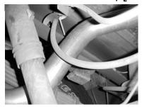
REMOVE THE REAR FACTORY HANGER. INSTALL HANGER #I TO THE BOTTOM STOCK HANGER HOLE. BOLT IT THROUGH THE 5<sup>TH</sup> HOLE DOWN FROM THE TOP OF THE HANGER. REPEAT ON THE DRIVER SIDE.
