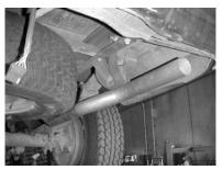
INSTALL OVER AXLE PIPE #D ON THE PASSENGER SIDE. NOTE: THE SPARE TIRE MAY NEED TO BE LOOSENED AND PUSHED TO THE REAR OF THE TRUCK TO GAIN TAIL PIPE CLEARANCE. OVER AXLE PIPES WILL BE PARALLEL WITH THE FRAME RAIL AND OUT APROXIMATLEY ½". USE CLAMP #G TO ATTACH PIPES D & E TO HANGERS #I
