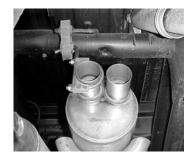
INSTALL HEADPIPES # A & # B USING CLAMP # G TO ATTACH HEADPIPES TO STOCK CONNECTOR PIPE. INSERT WELDED HANGER INTO RUBBER GROMMET. (DO NOT TIGHTEN).
