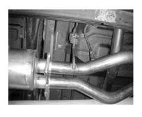
INSTALL HANGERS # J IN THE FRAME RATI APPROX. 18" FROM THE REAR OF THE FRAME. 10" METAL HANGERS ARE MOUNTED OUTSIDE THE FRAME. THE BOLT/WASHER GOES IN THE 3RD HOLE FROM THE TOP OF THE HANGER.
