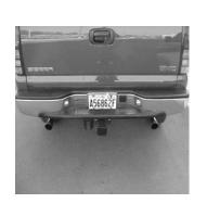
WHEN YOU HAVE EVERYTHING IN PLACE FIRMLY TIGHTEN ALL CLAMPS AND HANGERS. YOU MAY NEED TO USE THE SPARE TIRE BRACKET TO HOLD THE TIRE BACK. INSTALL IT 2" INSIDE OF THE UPPER SHOCK MOUNT ON THE DRIVER SIDE. USE ZIP TIES TO TIE AWAY BRAKE LINES. RE-INSTALL THE O2 SENSOR INTO PASSENGER HEADPIPE. USE ANTI-SEIZE ON ALL THREADS. INSTALL STAINLESS TIPS.
